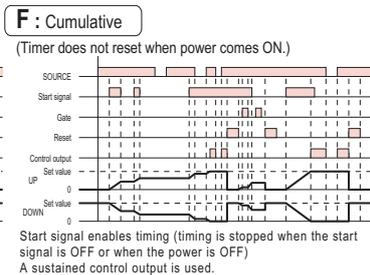
\*Note1. While the start signal is ON, the timer starts when power comes ON or when the reset input goes OFF.
