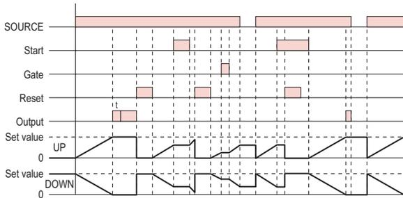
**Output mode A-3** : Power ON delay 2
