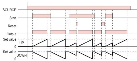
Output mode **D** : Signal OFF delay
