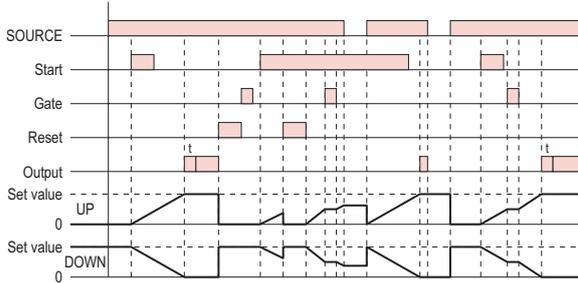
**Output mode A-1** : Signal ON delay 2
