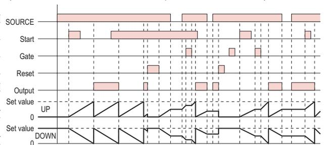
**Note.** In output mode A, A-1, A-2 and A-3, the control output is selectable between the sustained time period or one-shot time period.
