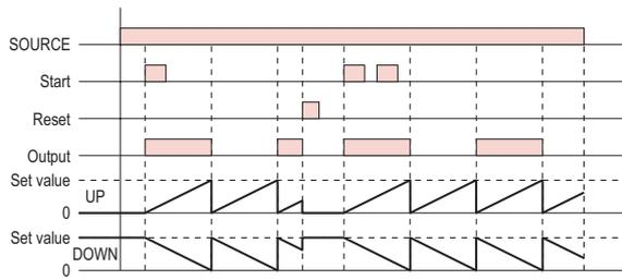
Output mode **C** : Signal ON/OFF delay
