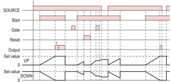
**Output mode A-2** : Power ON delay 1
