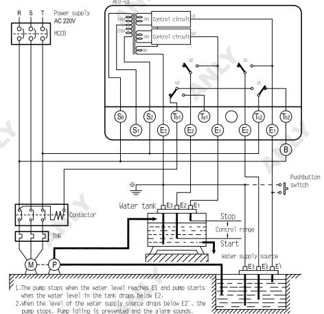
3 Insert a Pushbutton switch (NO contact) between E1' and E3 as shown by the dotted line. When starting the pump or after recovering from a power failure, if the water supply source level has not yet reached E1', press the pushbutton switch to start the pump by momentarily short-circuiting E1' and E3. When the pump stops during normal operation subsequent to an alarm issued for a low water level (e.g., the water level does not reach E2'), do not press the pushbutton switch.
