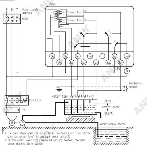
3 Insert a Pushbutton switch (NO contact) between E3 and E4. When starting the pump or after recovering from a power failure, if the water level has not yet reached E4, press the pushbutton switch to start the pump by short—circuiting E3 and E4. If the pump stops upon releasing the pushbutton switch, keep pressing the pushbutton switch.
